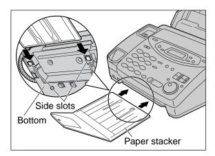
Confirm if the paper stacker is locked into the center slots.
